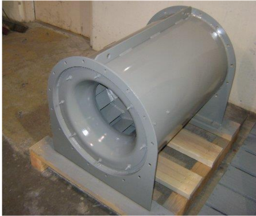
Typical In-Line Fan – Arrangement 4
